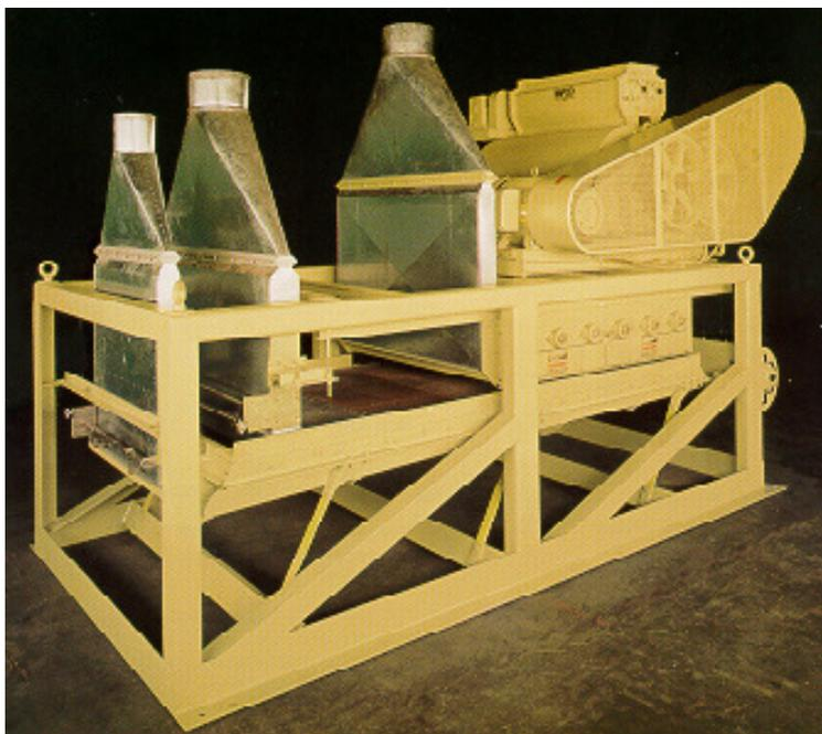
Decorticator with Hull Separator
