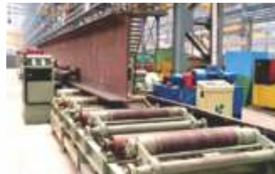
H-Beam Flange Straightening
