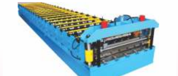
Roof Panel Roll Forming
