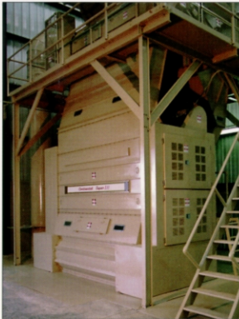
Inclined Cleaner over the Super III Stick machine with a 36" vacuum.
