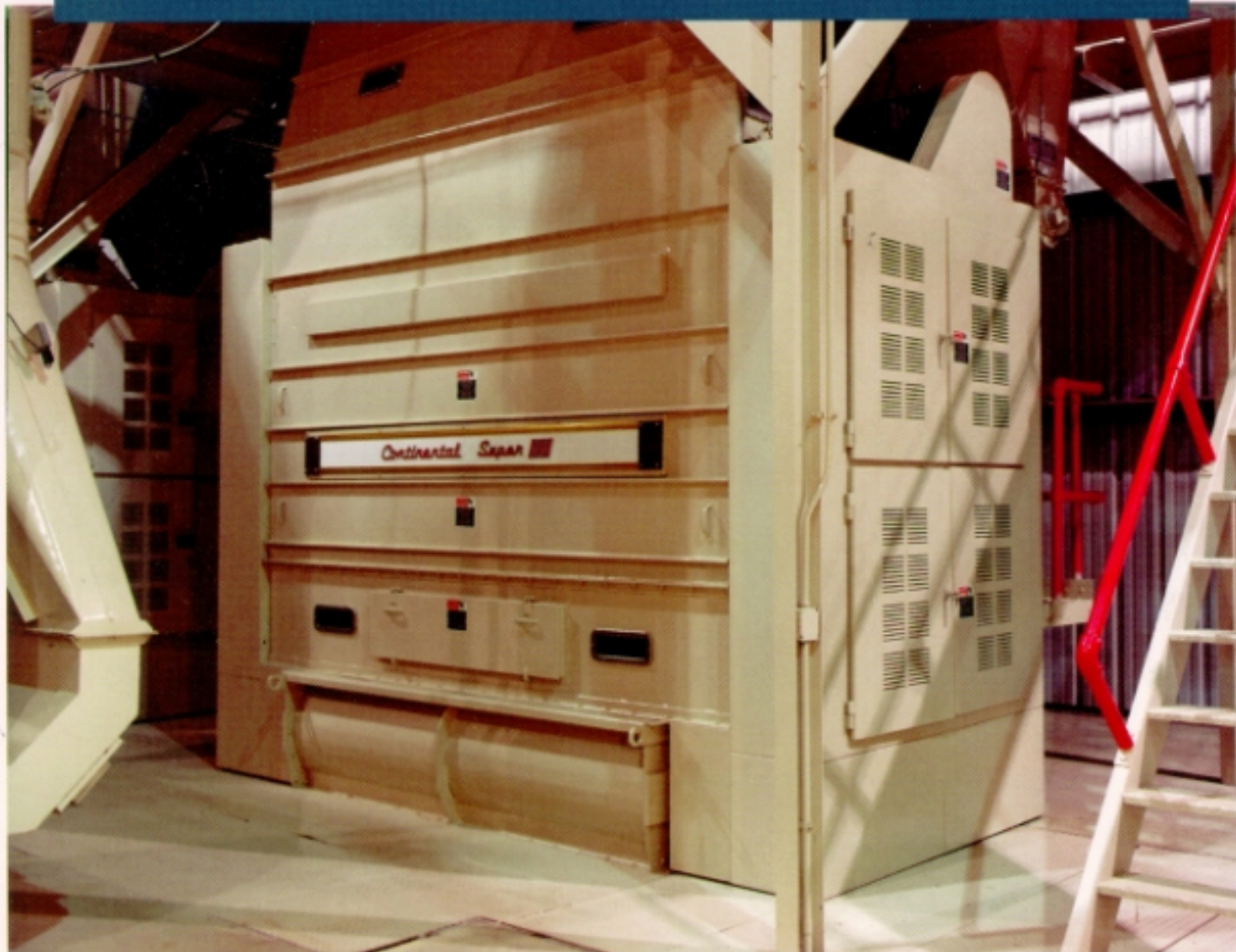
Shown with 24" vacuum - Vacuum, ductwork, and supports are not included with the Super III
