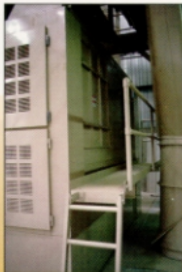
Wide rear access doors and catwalk.
