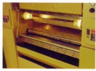
over the cleaning bars are reclaimed by a reclaimer saw and doffing brush. The doffing brush also doffs the cotton from the channel saw onto the cotton slide for delivery to the gin.
