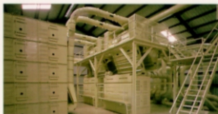
First Stage Cleaning Inclined Cleaners over Stick Machines
