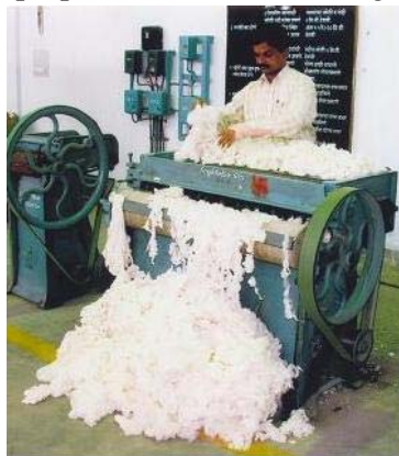
Figure Single Roller Gin
