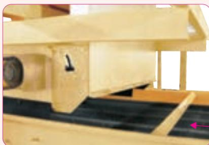
Top Tray from which Kernel (Meat) is being dispersed into the bottom right chute.
